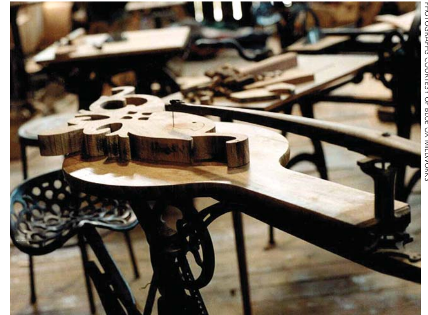
Not relegated to museum relics, Blue Ox uses its vast collection of antique machines to create quality millwork. Here is a gable in progress on the Barnes Velocipede Scroll Saw No. 2. Built in 1889, the saw contains a flat perforated belt and optional boring attachment.
